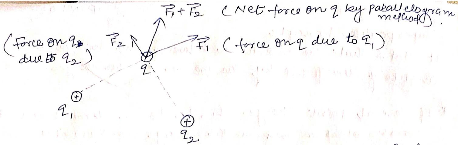
Two point charges  $q_1$  and  $q_2$  exert electric forces  $\vec{F}_1$  and  $\vec{F}_2$  on point charge  $q$ . The net force on  $q$  is vector sum of these forces.
